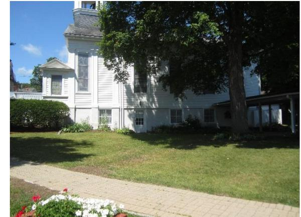
Stormwater is currently directed across the church’s lawn causing erosion issues. A rain garden adjacent to the building on that lawn can capture, treat, and infiltrate roof runoff. A preliminary soil assessment suggests that the soils have suitable drainage characteristics for green infrastructure.
