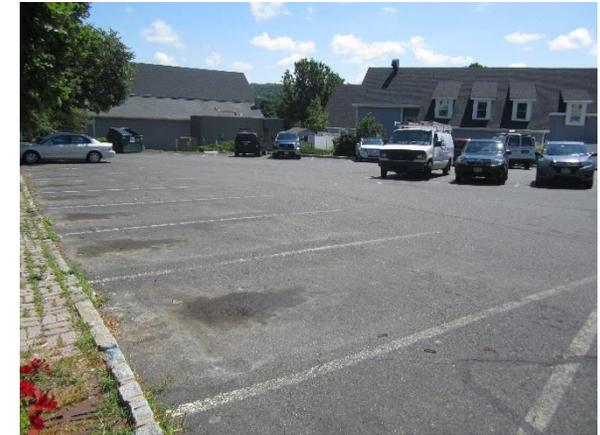
Stormwater is currently directed to an existing catch basin. Parking spots in the rear parking lot can be replaced with porous asphalt to capture and infiltrate stormwater. A preliminary soil assessment suggests that the soils have suitable drainage characteristics for green infrastructure.
